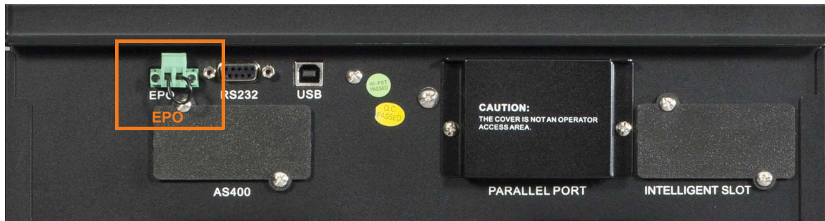
Figure 7.2 Emergency Power OFF
