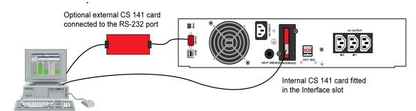
Simple Network Management Protocol (SNMP) is a world-wide, standardised communication protocol that can be used to monitor any network-connected device via a simple control language and display the results in a browser-based application. The software agent built in to the CS141 adapter card makes the UPS data available in this SNMP format which can then be utilized by a number of UPS management software applications.
