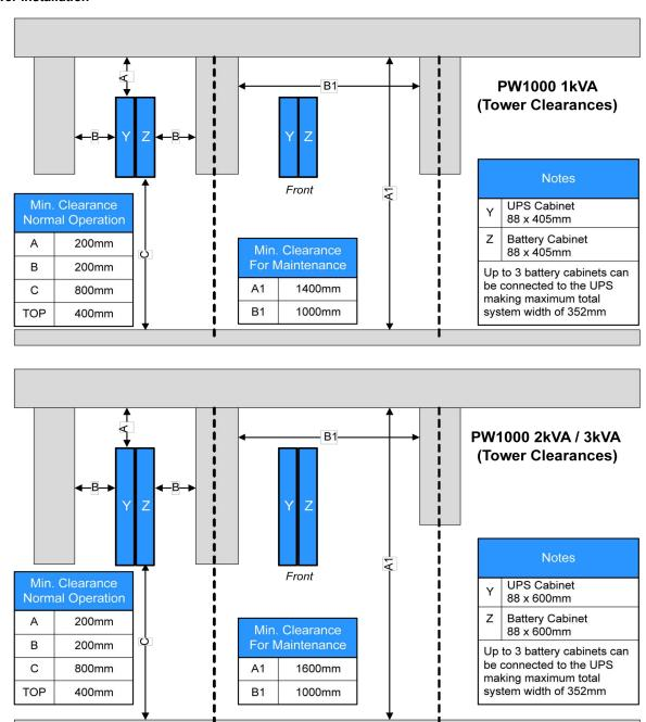
The total width of the system hardware can range from 88mm, for a stand-alone UPS cabinet, up to 352mm where the maximum of three (optional) battery cabinets are attached to the UPS cabinet – only one battery cabinet shown in the diagram above.
