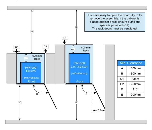
When the UPS is rack-mounted, a minimum of 200mm should be available between the rear of the UPS and the back of the rack cabinet to enable adequate ventilation and provide space for cabling. It is permissible to install the PW1000 1kVA model in a cabinet with a depth of 600mm, although this will only provide 195mm rear clearance rather than the desired 200mm shown in the above diagram.
