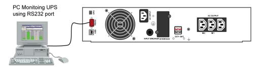
Note: The USB port is connected in parallel with RS-232 port and outputs the same data stream.
